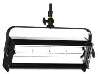
The Highlight LED utilises the best available remote phosphor technology and a unique optical design to give a bright and bold full spectrum 60° beam with excellent CRI and TLCI in 3200K, 4000K and 5600K. By using snap in phosphor panels you can swap colour temperature in a matter of seconds.
