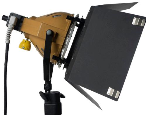
Controls on the lamp head are kept to a minimum for ease of use, and consist solely of a continuously rotating focus knob, with the on/off function being controlled from the 575-1200W Power Gems ballast. The ballast supports high speed work, up to 1000Hz operation. The ballast is wired with the standardized pin configuration.
